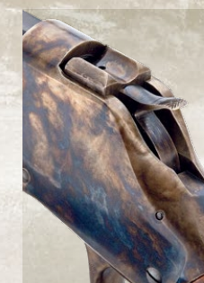
The 1885 High-Wall's loading lever (left), opens or locks the rifle's falling-block action (right).
